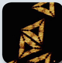
Triangle DNA origami structure imaged in fluid with ScanAsyst. Image size 300 nm. Sample courtesy of M. Endo and H. Sugiyama, Kyoto University.
