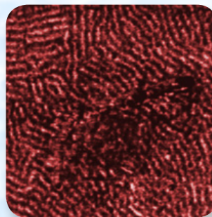
PeakForce TUNA current map reveals current paths in P3HT film. Image size 500 nm. Courtesy of P. Leclère, University of Mons, Belgium.
